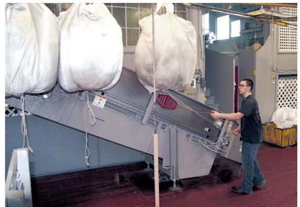
An ALADCO Linen Services worker prepares to open a sling and unload soiled goods onto the conveyor that feeds the company's new PulseFlow® continuous batch-washing system.
